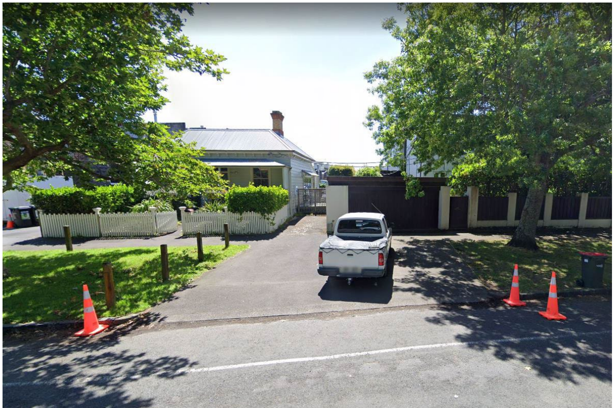
Figure 2: The existing shared vehicle crossing of 2 and 4 Hepburn Street (9m wide, to become 10.4m, widened on its southern side – where the bollards are. Note the hedge in front of the villa, 2 Hepburn Street, which is to be to a stipulated height to maintain visibility)
